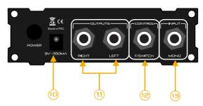
10 - DC PLUG - The DFX16 is connected to the mains using a 2-pole POWER connector jack. A matching mains adaptor is included with the unit.
