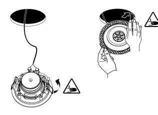
Lift the other clamp and insert in into the hole in order to set the loudspeaker in its final position.
