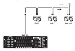
Connect fixtures using shielded 2-conductor twisted pair cable with 3-pin XLR male to female connectors. The shield connection is pin 1, while pin 2 is Data Negative (S-), and pin 3 is Data positive (S+).
